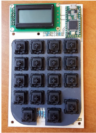
Figure 7: PCB with components soldered
